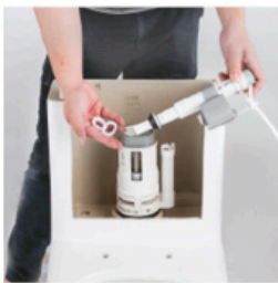
Unscrew the water inlet valve screw
